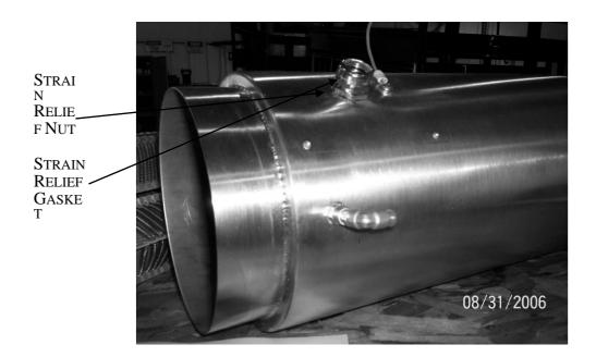
8. Note that the Y-shaped bracket is welded to the heater tube on the strain relief (wirebundle) end of the heater.
