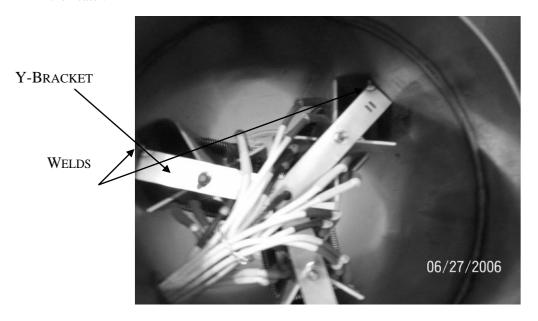
9. Remove the Y-bracket on the other end of the heater by removing the three (3) nuts and washers.
