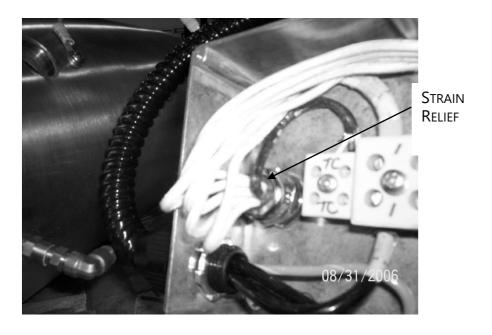
6. Remove the terminal box and mount by removing the screws holding the mount to the insulated heater jacket. Pull the wires through the terminal box.
