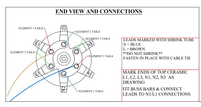
9KW 480V SINGLE PHASE UNIT - 76.8 Ohms PER ELEMENT / ZONE - 25.6 Ohms FINISHED. SUPPLIED WITH 2 x 30 AMP GLASS FIBRE LEADS 16" LONG
